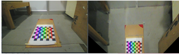
Figure 3: Left - Original image, Right - Inverse Perspective Transform (Bird's eye view)
