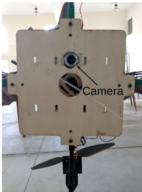
Fig. 17. The camera fixed on the tilt-augmented quadrotor.
