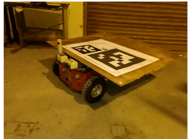
Fig. 18. Ground robot with the landing platform and the compound marker.
